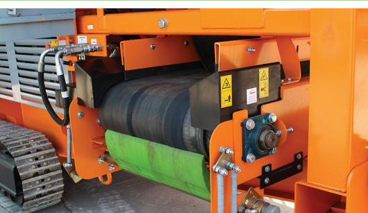
A destoning belt quickly separates rock and stone content from the finished product.
