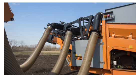
Any remaining contaminants are separated by triple suction fans, leaving a clean midsize fraction.
