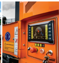
telematic monitoring system
