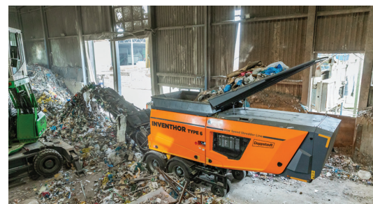
A hydraulically activated tipping hopper allows smart and efficient material feeding to the shaft.
