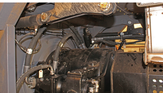
The VarioDirect drive allows the shaft to increase torque, reverse and start under load.
