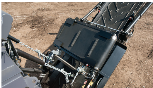
Recover metals and protect secondary processing equipment with a powerful neodymium magnet.
