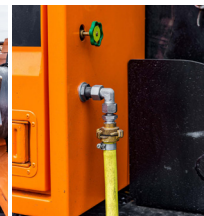
dust suppression system
