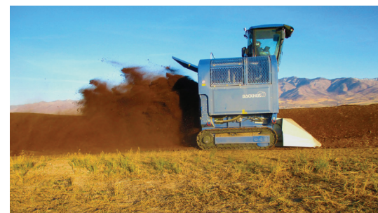
Independently controlled track clearers guide material to the drum and "float" to fit any pad.
